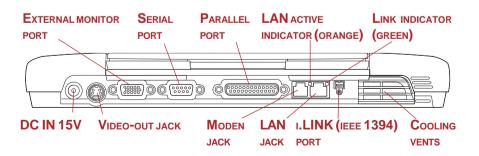
Figure 2-4 The back side of the computer
